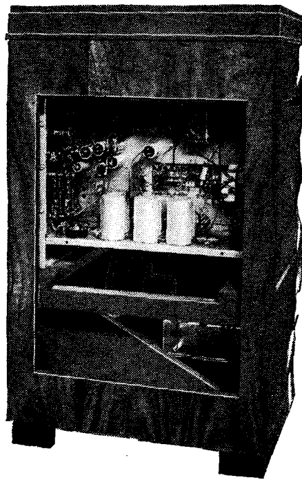
To provide good accessibility, the chassis of the R.G.D. Model 704 is mounted on its side, and is covered by an easily removable side panel.
